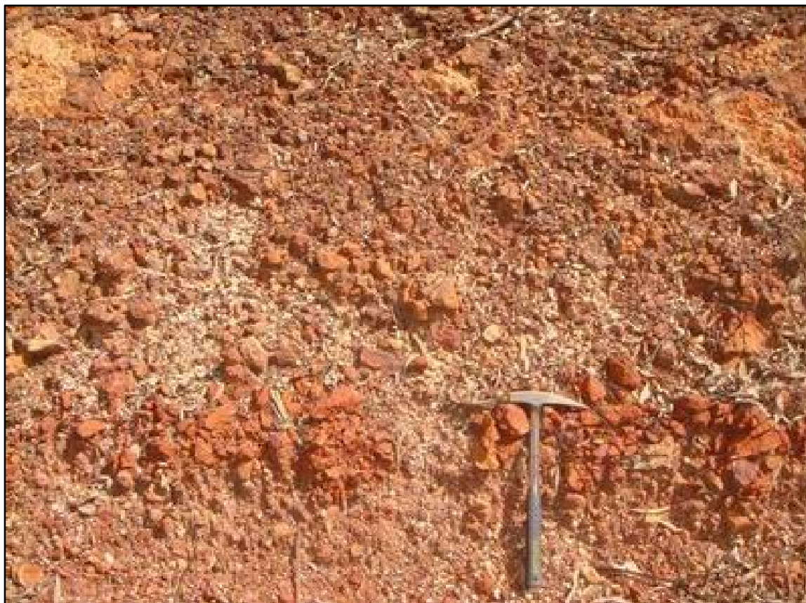
Figure 7: Extensive outcrop of ironstone 2-3m thick. Sample DR 4010, 35.7% Fe, 0.02% P
