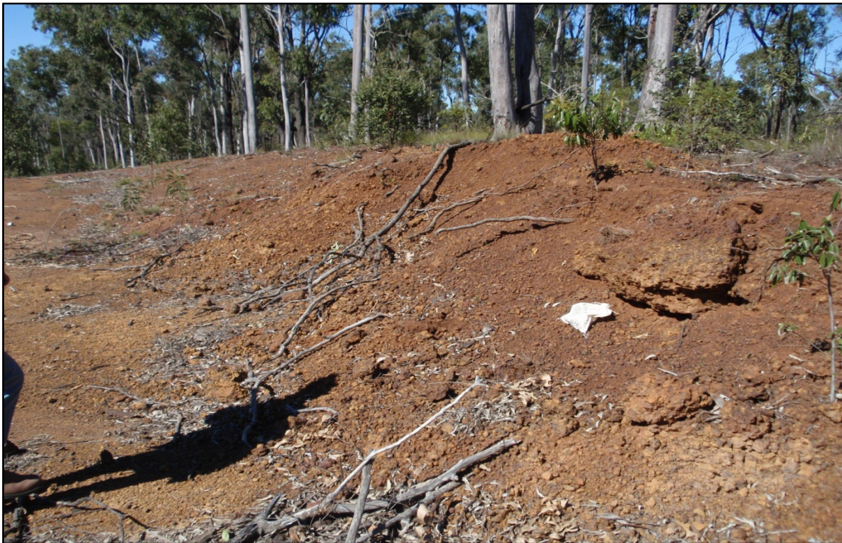
Figure 6: Outcrop of laterite iron – sample DR 2154, 49.9% Fe, 0.01% P
