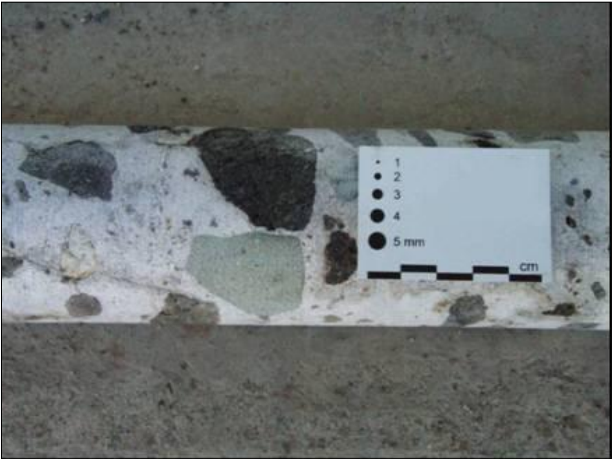
Figure 2: Mbetilonga Project - MBT003 and coarse angular basaltic-andesitic clasts hosted in well sorted sand to pebble sized limestone matrix.
